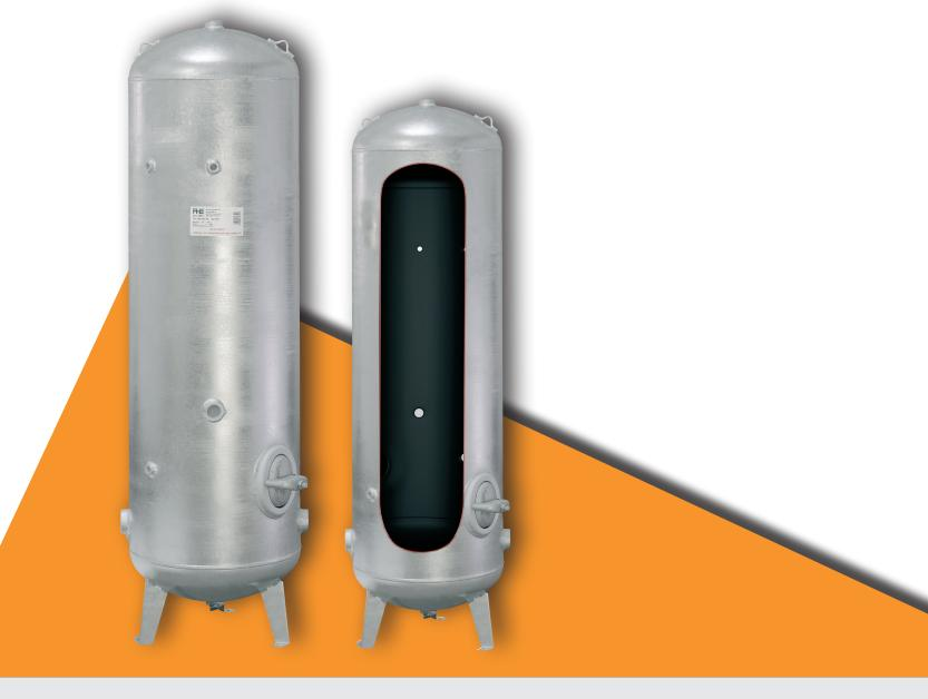
The pressurised water tanks of the WK type series are made of quality steel according to EN standards and are excellently suited for use in drinking and service water networks. The tanks with a capacity of 150 to 500 litres are particularly well suited for damping pressure surges in networks or for maintaining a constant power pressure.
